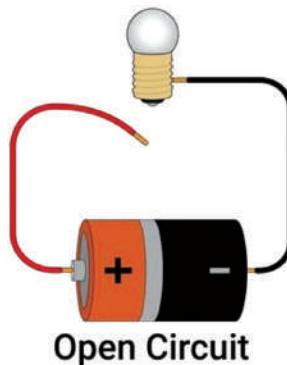
Observe the image. See that the circuit is open, and the path is incomplete where the red wire is not connected to the battery and only the black wire is connected to the Battery. Therefore, due to the incomplete circuit, electricity does not flow, and the light bulb will not glow.
