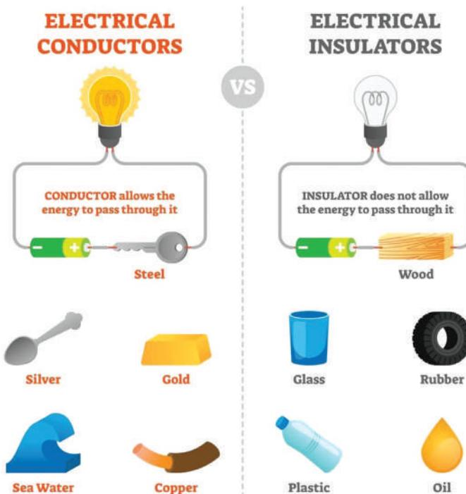
Conductors are surrounded by insulators to prevent electrons from escaping.
