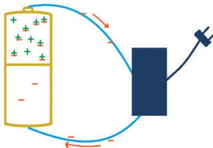
The charger uses electricity (usually from a wall socket) to force electrons to flow in the direction they don't want to go.
