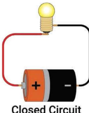
Observe the image. See that the circuit is closed, and the path is complete between the positive and negative terminals of its power source. Therefore, due to the complete circuit, electricity flows smoothly and the light bulb shines brightly.
