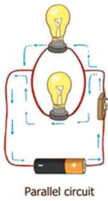
In the image shown above, Bulb 1 and Bulb 2 are connected to the circuit in parallel. So, when current flows, it gets distributed into two branches and only some amount of current flows through all the two bulbs of the total current.
