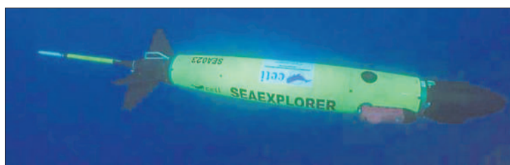
Project CETI's Glider, a whale communication data collection technology, is deployed in the Caribbean Sea off Dominica
